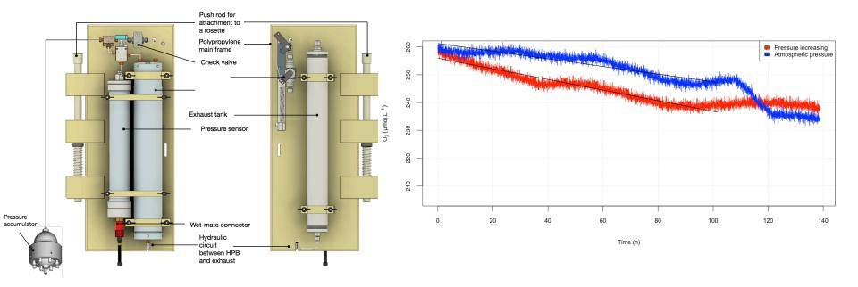
HPSU : a new and commercially available device to perform high-pressure sampling
