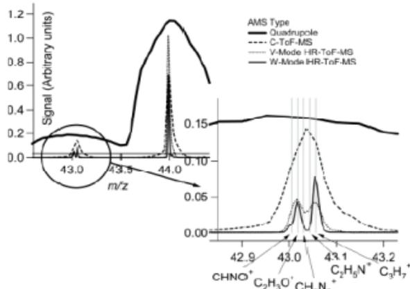
**Figure 3.** Peak comparisons for the four versions of the AMS. Resolution improvements are obvious in the progression from Q-AMS to C-ToF-AMS to V-mode to W-mode of the HR-ToF-AMS.
